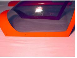
☐ Install the canopy using the small wood screws. If satisfied with the fit, remove the canopy and hatch and wick a small amount of thin CA into each of the screws holes on the hatch. Once dried, reinstall canopy with optional canopy glue if desired. Caution! CA will fog the canopy if installed before completely drying.
