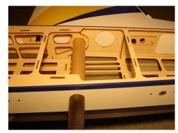
Tip#8 If the wing is tight you can coat the tube with a little baby powder to aid the insertion of the wing panels.
