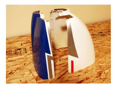
We have provided a split cowl with your Edge. This allows better baffling setups as well as making it easier when installing a DA-200. Always wear a mask and eye protection while cutting fiberglass. Take your time while installing the cowl. With care you will end up with a professional installation that will make an impression at the field.
