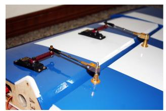
Be sure that you install the horns at the same height from the hinge line (see attached). By doing so you will have very little servo matching to do afterwards.
