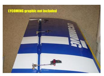
Screw in four HD ball links onto the counterclockwise ends of the 2.5" H9 push rods and screw the other end into the control horn. Ensure everything is still centered. Don't forget to add locknuts to the 4/40 bolts attaching the ball links to the arms.
